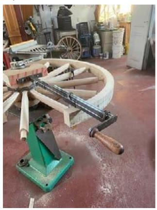
Once both felloes were installed, I moved the wheel to my tire table and tightened it all together with an adjustable clamp to test the fit and the dish. My wheel table has a 3/4-inch vertical rod to tighten the wheel. The centre circle that is cut out to allow for the depth of the hub can move up and down on the threaded rod, so by combining the round clamp with the adjustable hub support, I can set the desired dish exactly before installing the tire.
