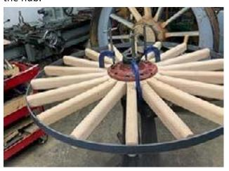
I do not see many Archibald hubs in my shop, so had to make specific hoops to hold the spokes in place while the hubs were drilled. Once I had the spider assembled, the rest was relatively straightforward until it came to sizing the tires.
