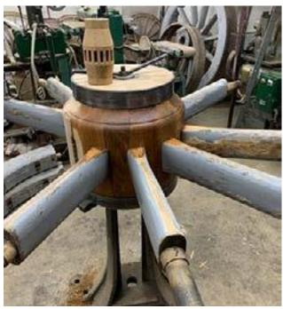
There were a few spokes that were not useable which had to be matched exactly. The felloe tenons were stepped to add to the complexity, so it was back to my trusty lathe to produce the exact replicas.
