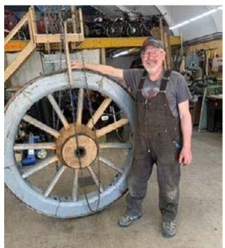
In addition to the heavy canon wheels, a pair of relatively heavy wagon wheels came in to be rebuilt. This was slightly unusual as they were Archibald wheels.
