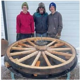
After adding tire bolts and custom made felloe plates, I tested it for the proper fit before painting and final installation.
