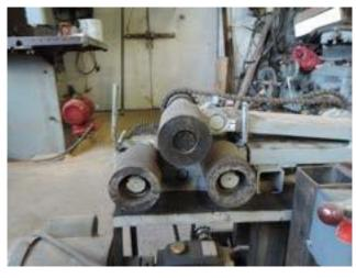
The bending pressure is provided by a threaded rod that connects the swing arm trunnion to the main body trunnion. Rotation of the rod opens or closes the gap between the drive rolls. The main body is made from  $1 \times 4$ -inch bar stock for the sides and  $3/4 \times 8 \times 18$  inches for the base.
