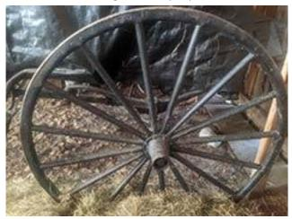
While the tires show significant wear, the goal would be to keep them, realizing that if the buggy were to be actually used, they would have to be replaced. These are Sarven hub wheels, measuring approximately 39" and 43" diameter minus the tire. The original fellies are 1 1/2" deep by 1 1/4" wide. Sarven spokes are 1 1/4".
