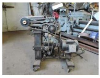
The bottom half is made from 1 1/4 x 4-inch bar stock 18 inches long, with ears to capture the hinge pin. The complete swing arm assembly is fixed to the main body by four 7/16-inch bolts which pass through spacers. This arrangement allows for adjusting the alignment of the rolls.
