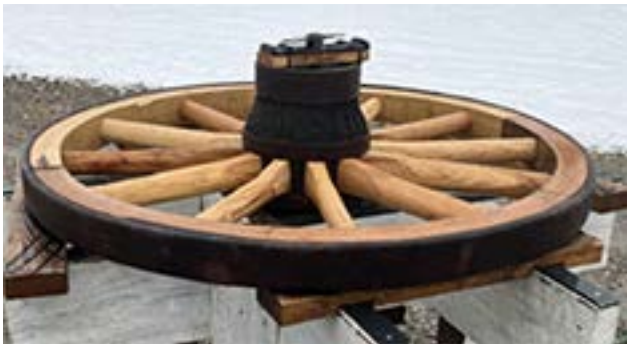
After shrinking the tyre on.
